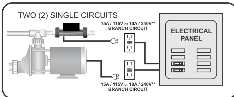
**\*\*240V Heater cords do not have a Nema plug and require hard wiring of the unit.**
