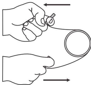
**Note: Let the saw blade do the work, do not put excess pressure on the plumbing. Have someone else stabilize the plumbing while you cut if needed.**
