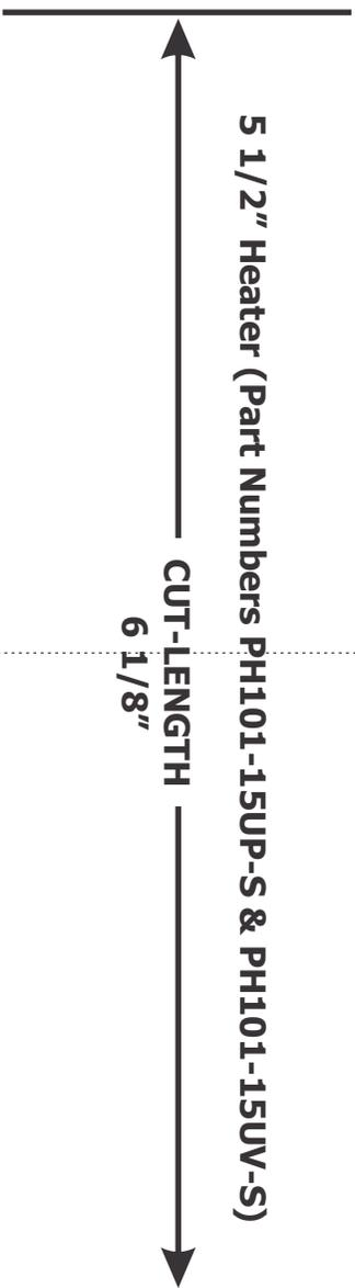
Use this template as a guide when making cuts during Whirlpool Bath heater installation. **Cut and detach from instructions.**
